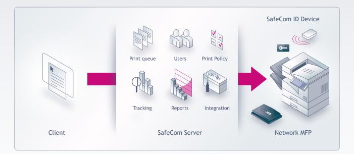
SafeCom Controller provides secure printing and access control - users send their print and then authenticate at any SafeCom-enabled network MFP or printer to retrieve it. Authentication using cards requires an ID Device.
